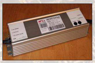
This slim and light outdoor power supply is suitable for various VSAT applications, which require 48 VDC output and 90-264 VAC input. The unit is equipped with short circuit, overload, over voltage, over temperature protection and certainly is in compliance to worldwide safety regulations.
